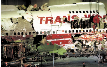
Debris from TWA Flight 800 was pieced together following the fatal crash of the Boeing 747 in 1996. Government investigators concluded that the likely trigger was a short circuit from damaged wiring—wiring “not atypical for an airplane of its age.”
