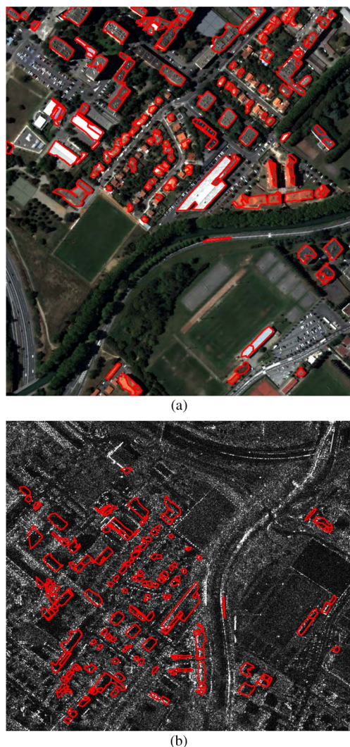
Fig. 10. Building detection without DB: building outlines projected (a) on the optical image and (b) on the SAR image.
