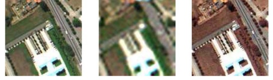
Fig. 2. (Left) Reference image. (Middle) HS image. (Right) MS image.
