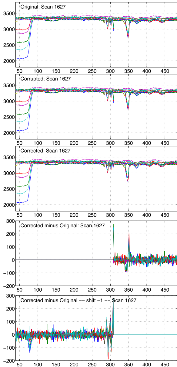
Fig. 8. Scenario 1: End of scan #1627 appears as badly corrected due to extra detected glitches, which results in the deletion of an entire frame. Note that the overall behavior of the individual signals in each channel has been preserved after correction (no channel permutation).
