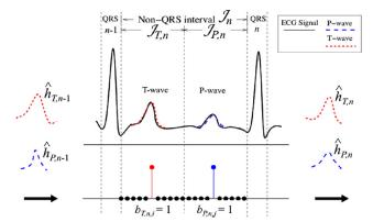
Fig. 1. Signal model for the beat-to-beat processing scheme.
