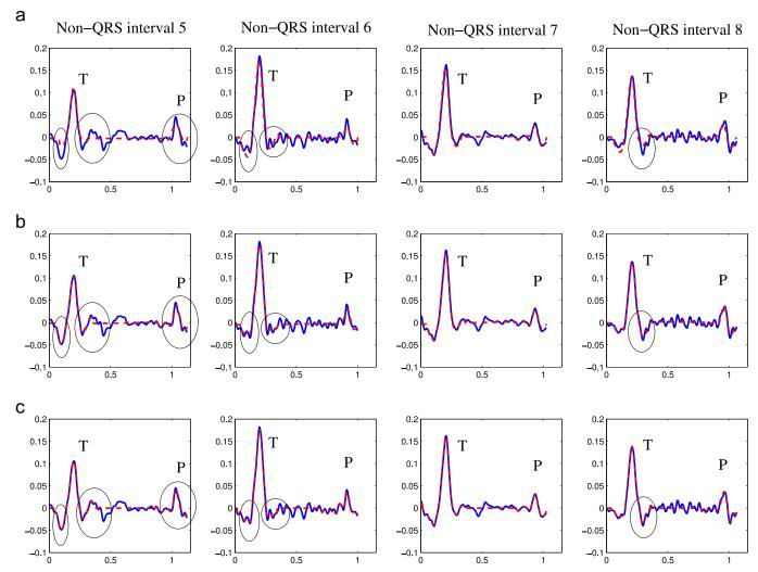
**Fig. 5.** Four other consecutive segments from QTDB dataset sele0136 (blue) superimposed with their reconstructions using the estimated parameters (dotted red). (a) PCGS multi-beat method of [10]; (b) proposed beat-to-beat BGS method; (c) proposed beat-to-beat MPF method. (For interpretation of the references to color in this figure caption, the reader is referred to the web version of this article.)
